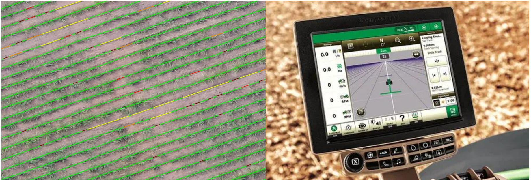
Figure: Example of crop-row identification performed manually by an expert (left). Example of an autonomous machinery it is being guided by the detected crop rows. CommandCenter™ Premium produced by John Deere, extracted from https://www.agriexpo.online/prod/john-deere/product-169419-2710.html
