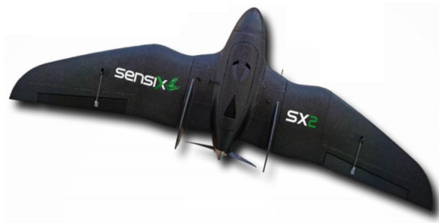
Figure: fixed-wing UAV SX2 made by Sensix Innovations and responsible for capturing the imagery used in this work.
